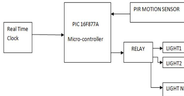
**Figure 4: Block Diagram of Occupancy Sensing Module**
