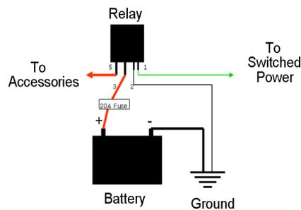
**Figure 7: Circuit Diagram of the Relay Circuit**
