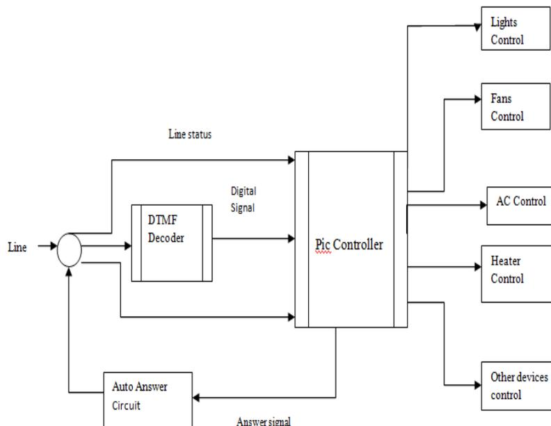
**Figure 5: Block Diagram of the DTMF Based Electric Control System**
