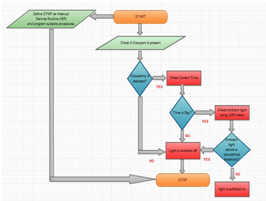
Figure 6: Flowchart Showing Algorithm Used in the Proposed System
